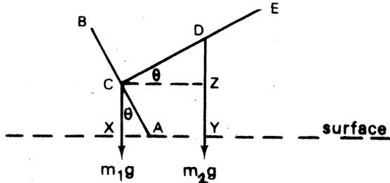
Let  $CA = d_1$ ,  $CD = d_2$ , mass of head =  $m_1$ , mass of pointer =  $m_2$  and angle  $ACX = \theta =$  angle  $ZCD$ . The pin will return to the point down position if:
